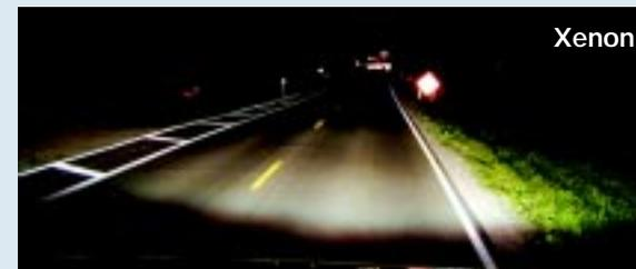
*Xenon produces up to 70 percent more light output and a wider beam which potentially increases safety.*
