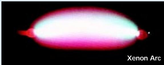
encased in a special glass jacket that filters the light to eliminate harmful ultraviolet rays. The light is emitted by an electrically energized gas — a plasma discharge — formed and sustained between two electrodes.
