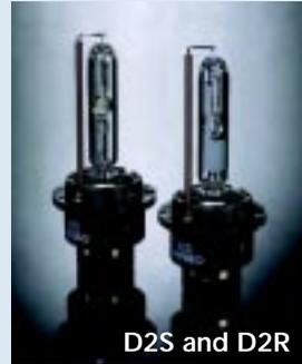
Two lamp types are offered: D1 lamps with an integrated starter and D2 lamps with a plain plastic base. In both, there is an S-type specifically designed for projector optics and an R-type for reflector optic systems. The Xenon system includes an electronic ballast that controls the arc ignition process and sustains the arc in normal operation.
